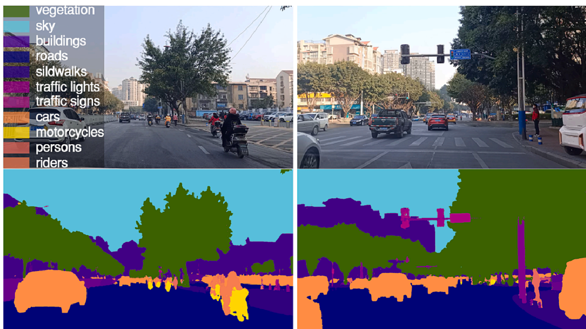
Fig. 3. Two examples of extracted images and semantic segmentation result.
